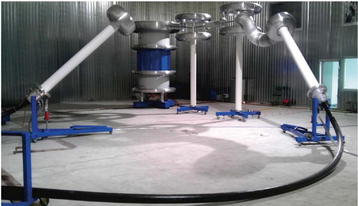
The cable termination requirement is very high for testing 66kV or above XLPE cables.
